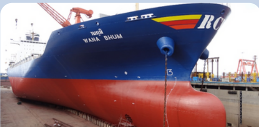
RCL ships use Antifouling paint without cybutryne. The absence of Cybutryne helps reduce its impact on the environment and aquatic animals as Cybutryne can have adverse effects.
