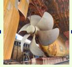
An energy-saving device attached to the propellers to break up the hub vortex or swirls generated behind the rotating propeller, resulting in a reduction in fuel consumption.
