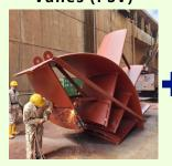
An energy-saving device for full-form slower ships enabling significant power savings at a given speed or for the vessel to travel faster at a given power level.
